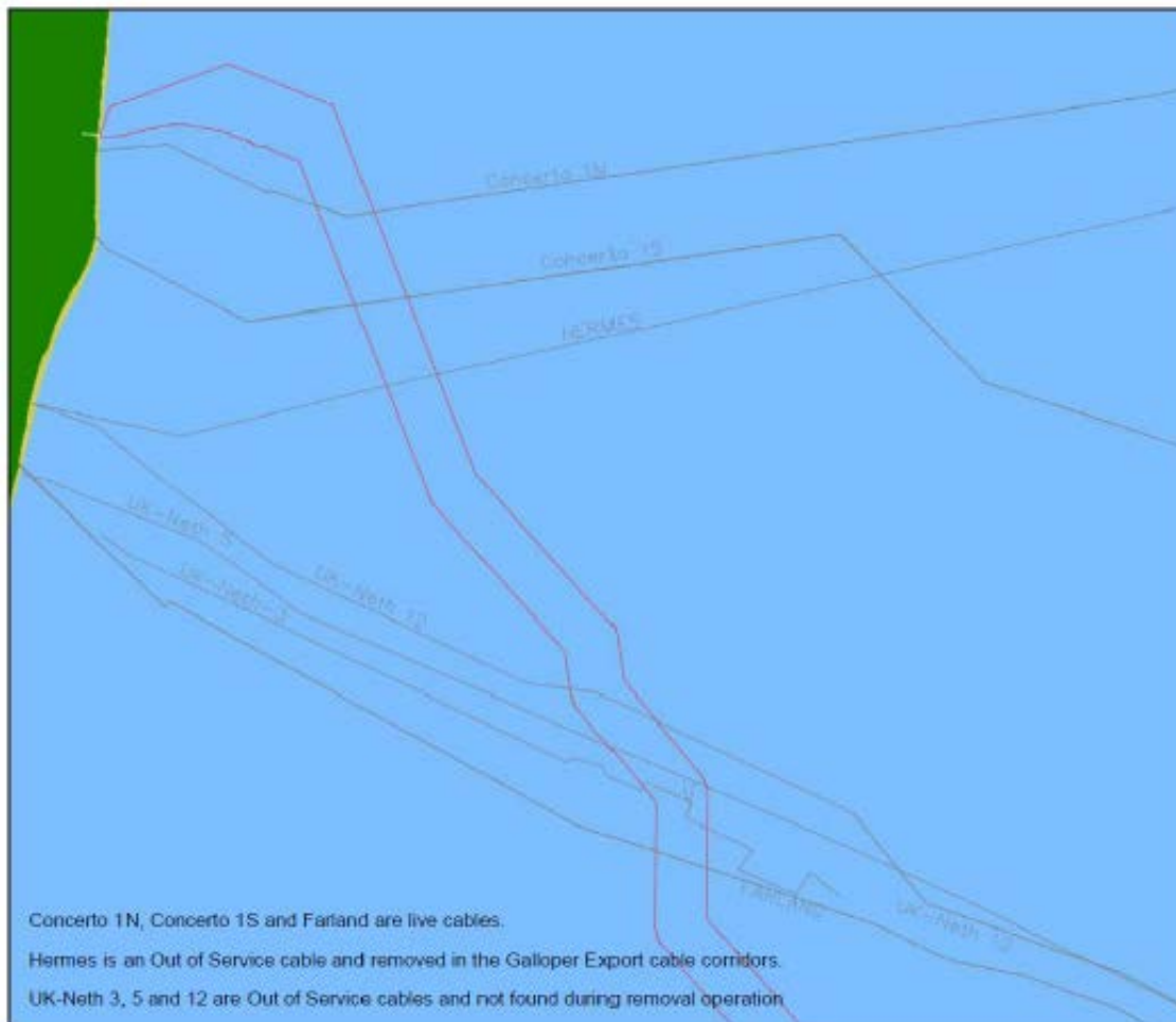
Figure 3.8: Cable Crossings along The Export Routes
